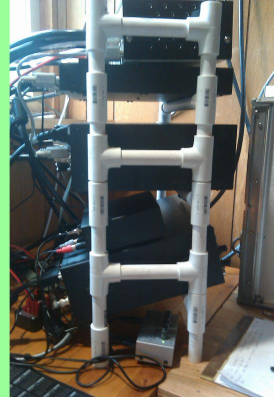
PVC Rack Mount Can be spun around to work on cables.
